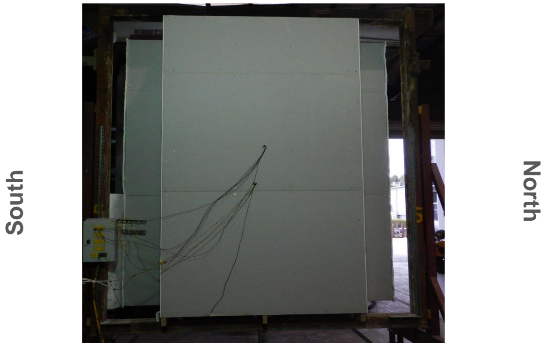
Figure 9 Unexposed face of the specimen before the start of the test
