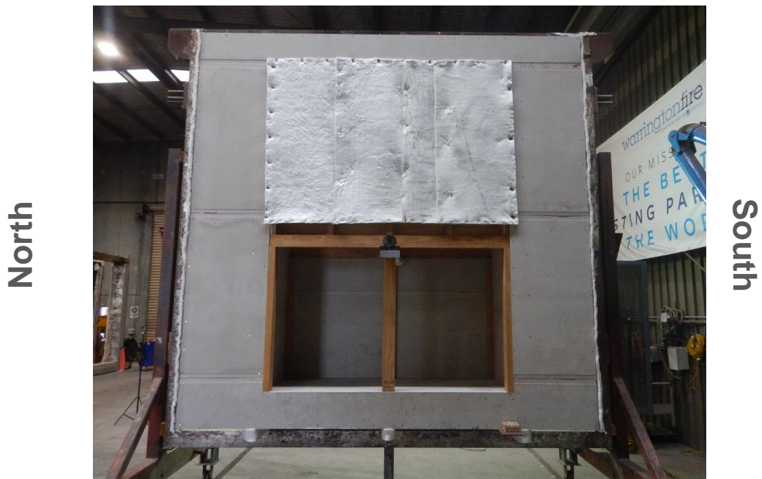
Figure 10 Exposed face of the specimen before the start of the test
