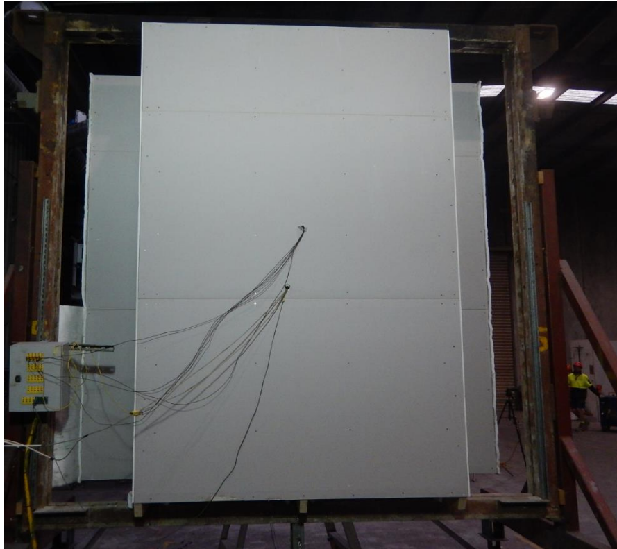
Figure 11 Unexposed face of the specimen at the end of the test
