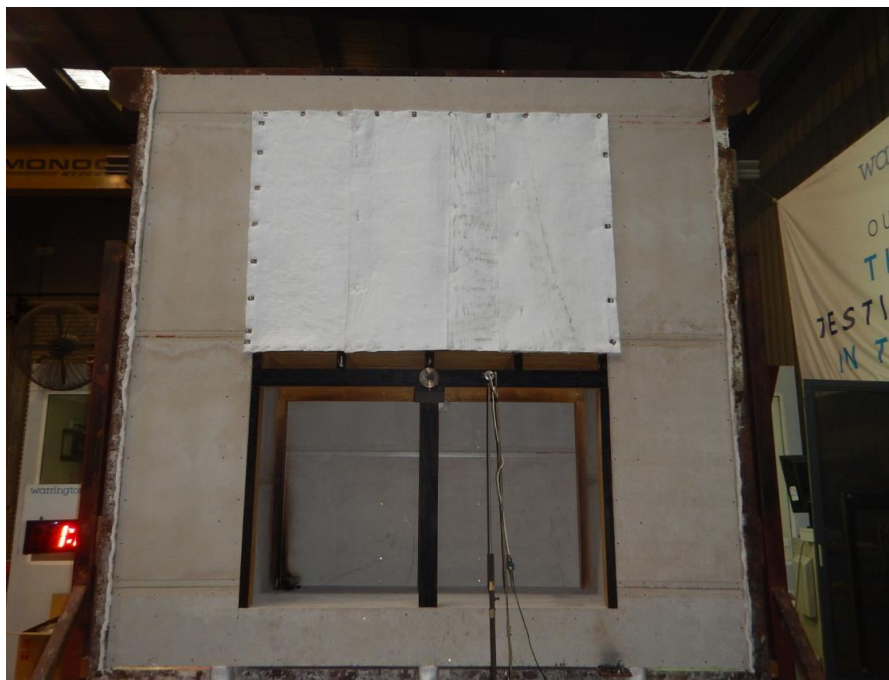
Figure 11 Unexposed face of the specimen at the end of the test
