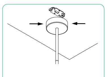
Screw canopy of light fitting over bracket, using the two screws provided.
