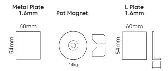
Wall Pot Magnet Install Metal Plate
