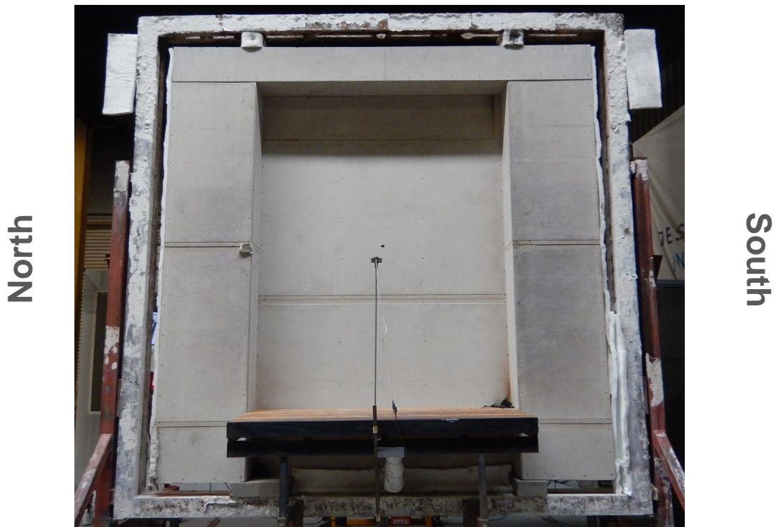
Figure 14 Exposed face of the specimen at the end of the test
