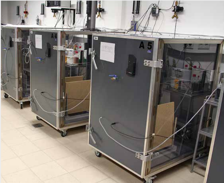
Test chambers with a volume of 1m 3 at Fraunhofer Institute WKI.
