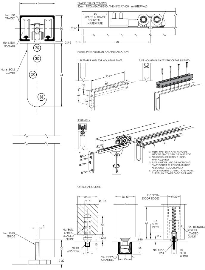
\* WHEN USING No. 100SCT SOFT CLOSE, No. 100 TRACK MUST BE ANODISED 620 MIN PANEL WIDTH SINGLE SOFT CLOSE, 820 MIN PANEL WIDTH DOUBLE SOFT CLOSE
