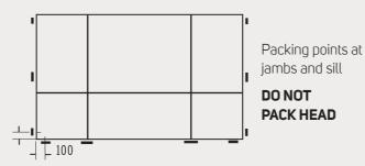
• The frame must be square and out of twist which is essential for the smooth operation of the sashes.
