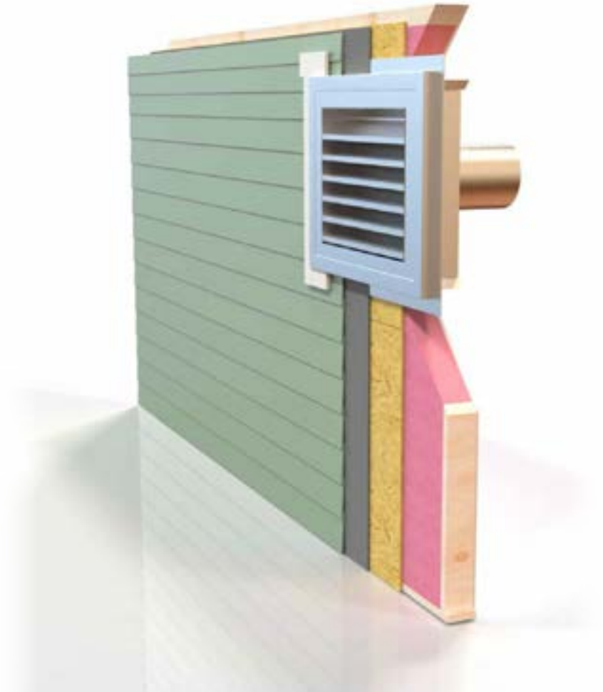
Horizontal Termination (Inline Power Exhaust Fan)
