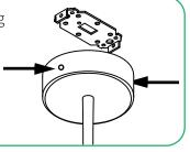
Once hung, screw the globe in, making sure to place the 40mm finishing cuff over the base of the lamp holder to conceal componentry.
