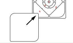
Push the inner corner of the leaf through Hole B in the suspension plate, ensuring a snug fit with no gaps.
