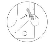
Pull out the two transit rods located below the two lower transit bolt holes.
