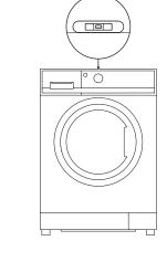
Move the washer into its final position allowing for required clearances.
