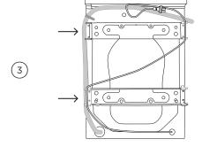
Detach the drain hoses from the plastic clasp, and remove the clasps on the side of the transit braces.
