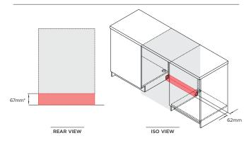
Service outlet at rear extends both sides, hoses and cords can be routed to either or both sides.
