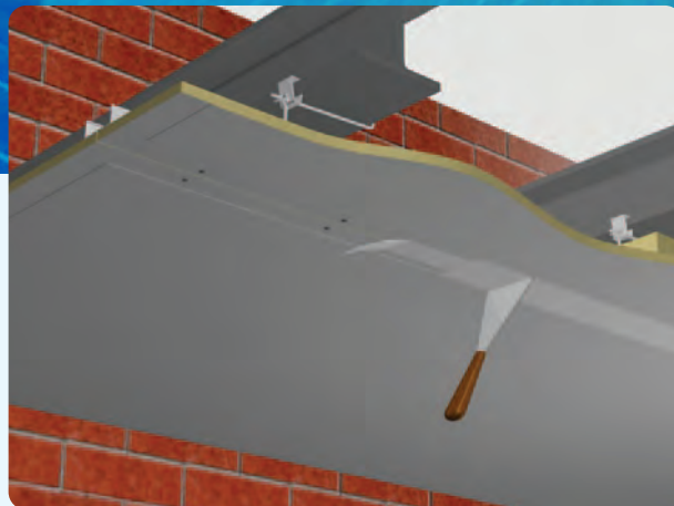
Gaps between boards and their covering
