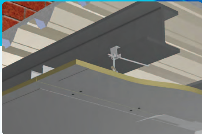
Screw assembling, spacing 250 mm
