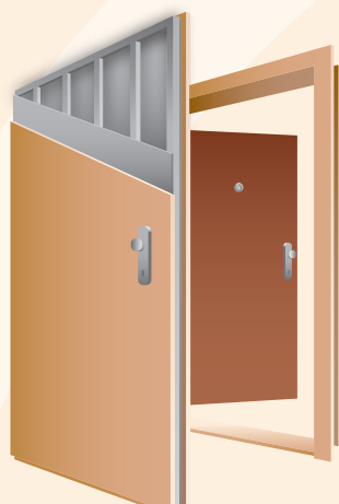
Construction of fire-resistant door
