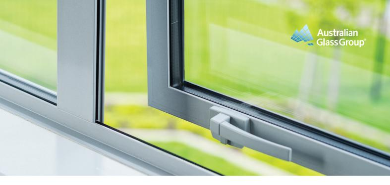
Insulglass<sup>®</sup> Insulated Glass Units (IGU) consist of 2 or more pieces of glass manufactured as one unit with a trapped air gap separated by a desiccant filled spacer bar and sealed with a primary and secondary seal for structure and guaranteed performance.
