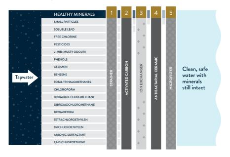
Note: Premium cartridge filtering shown. Different substances are filtered depending on the cartridge type used. Based on Japanese Industrial Standard JIS S 3201.
