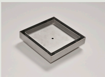
Standard Tile Insert Drain Suits tiles up to 12mm 130mm x 130mm 23mm Deep DN80
