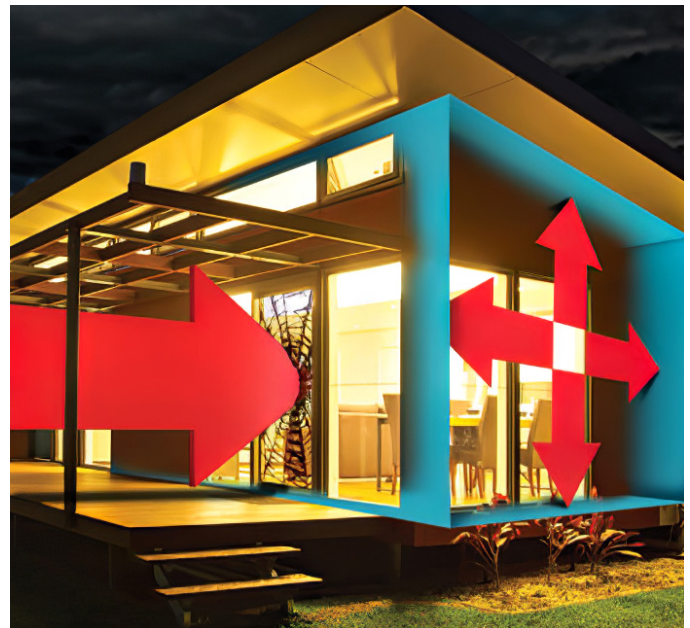
Positive Internal Pressure Windows breached, structural integrity compromised.
