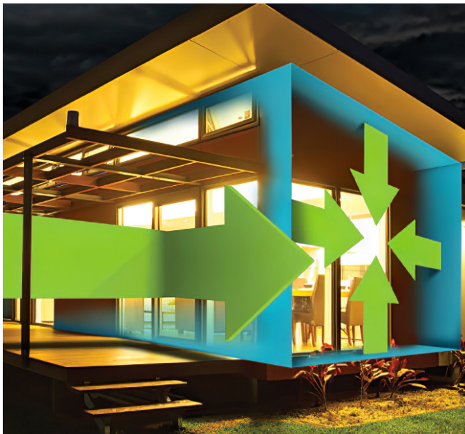
Negative Internal Pressure Windows intact, building remains structurally safe.
