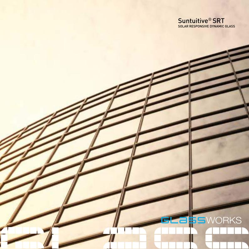
Australia's first Solar Responsive Thermochromic (SRT) Glass, Suntuitive® is a dynamic thermochromic technology incorporated into a PVB interlayer that causes the glass to adjust the light transmission and heat gain properties based on the intensity of the sun. As the sun strikes the window, it absorbs and adapts the tint - optimising daylight and reducing heat gain and air-conditioning loads.
