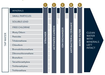
Note: Premium cartridge filtering shown. Different substances are filtered depending on the cartridge type used.
