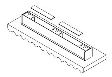
Remove aluminium plates from rear of LED base.
