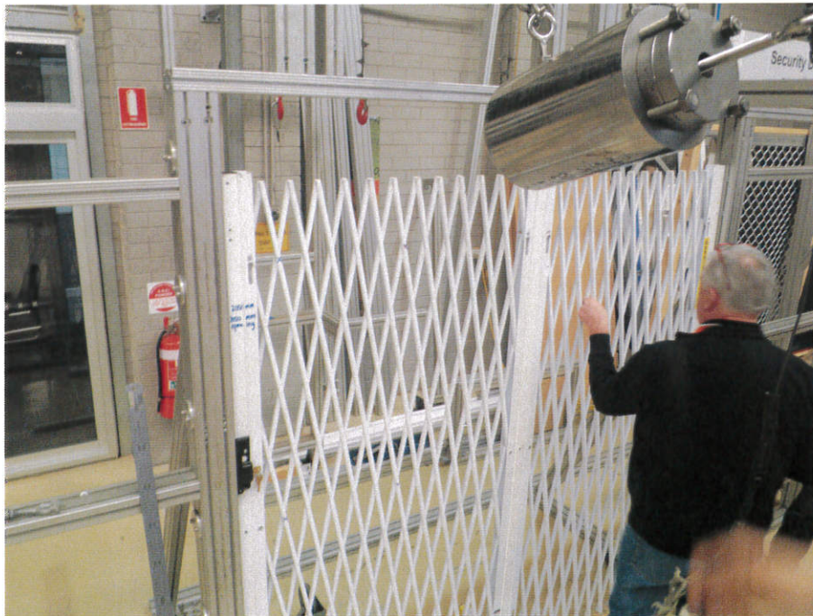
Figure 3: Impactor set up to hit top left corner with 150 J
