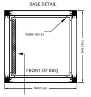
BRING UNDERGROUND SUPPLY PIPES/CABLES UP TO THE LEFT SIDE OF HOTPLATE OPENING LOOKING FROM THE FRONT AS INDICATED BY SHADED AREAS. DO NOT BRING PIPES/CABLES UP DIRECTLY UNDERNEATH HOTPLATE AND ENSURE PIPES/CABLES DO NOT RUN UNDERNEATH HOTPLATE.
