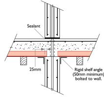
NOTES: 1. Standard end bearing of **Stramit Condeck HP®** Decking is 50mm. 2. For 25mm end bearing, end of sheets must be fastened to support.
