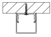
Prior to installation apply a bead of adhesive to the internal face of the step in the cover (as shown in DETAIL A) and click over the base. Ensure that the cover is secured in place until the adhesive sets.
