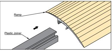
**STEP 3 -** Finally insert the ramp and joiner into the base.
