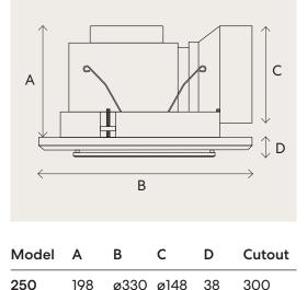
The Hybrid range is a high quality modern ceiling exhaust fan that can be connected to 150mm ducting. The Hybrid comes with a built in backdraft shutter and is available with either a round or square fascia. The fan comes with a lead and plug for easy DIY installation.
