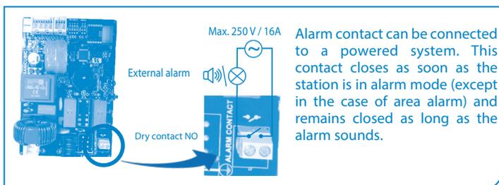
Alarm contact can be connected to a powered system. This contact closes as soon as the station is in alarm mode (except in the case of area alarm) and remains closed as long as the alarm sounds.
