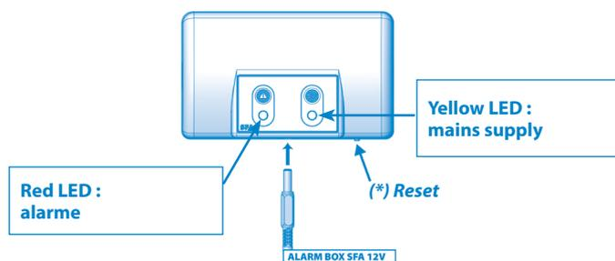
1/ The red general alarm LED reproduces the operation of the corresponding LED on the SANICUBIC® control panel. The alarm unit sounds as long as the fault is present. To stop the alarm, press the reset (\*) button on the device's keypad or the button under the alarm unit.
