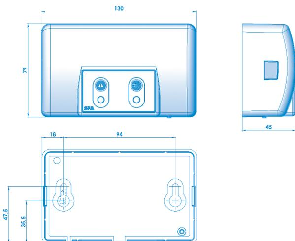
The **SANICOM®** alarm unit does not require a separate power supply. The power is supplied through the **SANICOM®**. In case of power failure, the alarm unit's battery takes over.
