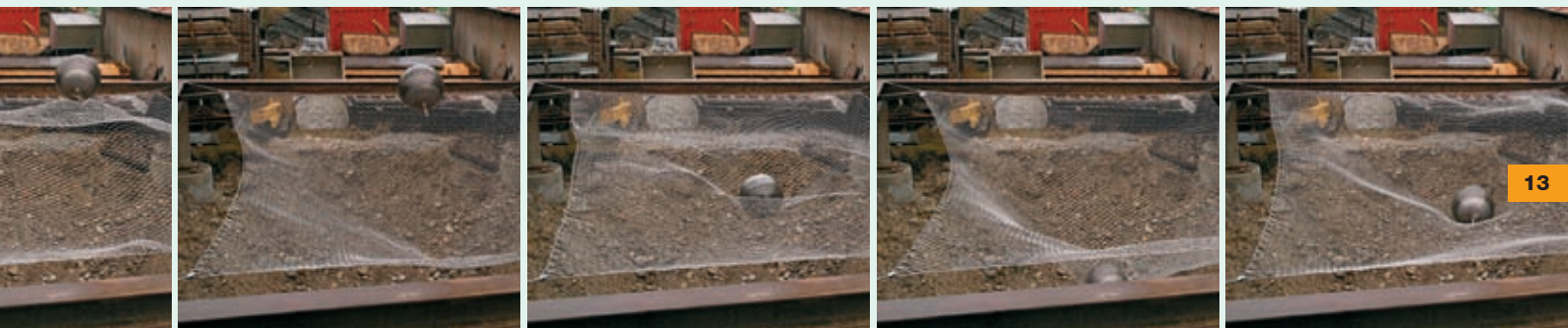
Webnet with extended mesh angle: when stretched, the wire ropes load the sleeve (breaking limit).
